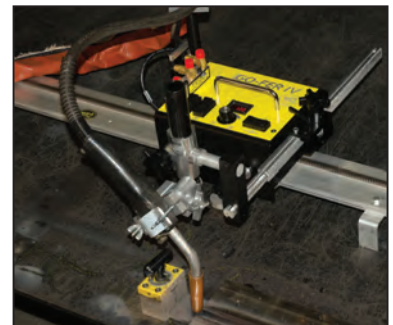
Shown above, welding setup of Go-fer IV
