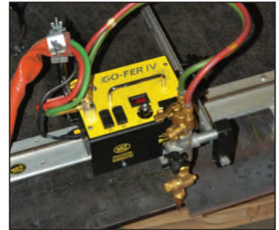
Shown above, oxy-fuel setup of Go-fer IV
