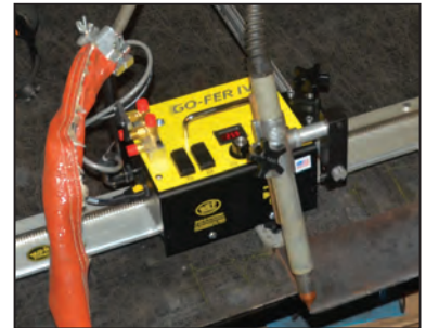
Shown above, plasma setup of Go-fer IV
