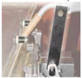
MSQ-165 ON/OFF Magnetic Stop for limit switch activation
