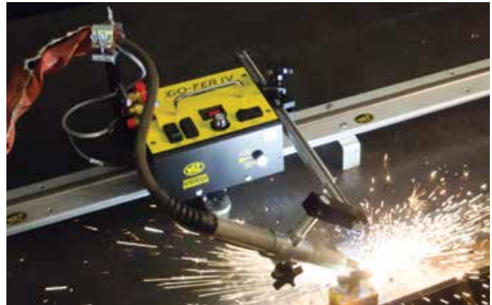
Shown above, plasma setup to perform back gouging
