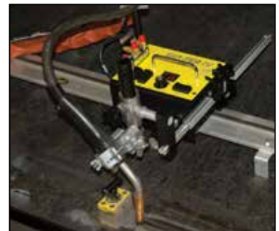
Shown above, welding setup of Go-fer IV
