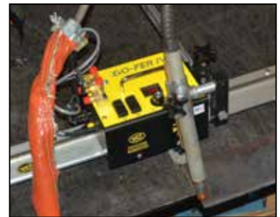
Shown above, plasma setup of Go-fer IV
