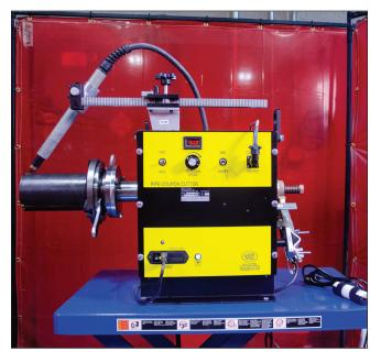
The **PCC-3** Pipe Coupon Cutting Machine is used for cutting pipe to a desired length or for beveling the edge of a pipe for weld preparation and is designed to be fixed to a worktable. It is bolted to the table through mounting holes located in the legs of the machine.
