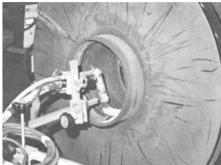
Bug-O System providing automatic arc translation.
