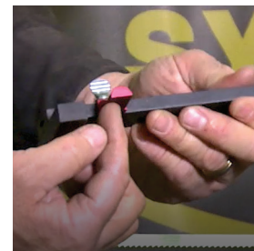
Closeup Side View of Torch Clearance Gauge
