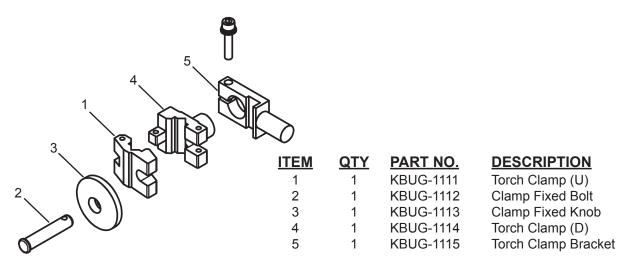
Note: KBUG-1100-1 Torch Holder can be used instead of a KBUG-1100 Torch Clamp Assembly.
