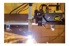
For metal workers who need to easily and repeatably bevel or vertically cut metal, the DC-IV MAX is a unique turnkey solution that combines a purpose built tractor and controller from Bug-O Systems® with a Powermax® series or MAXPRO® plasma cutting system from Hypertherm®.
