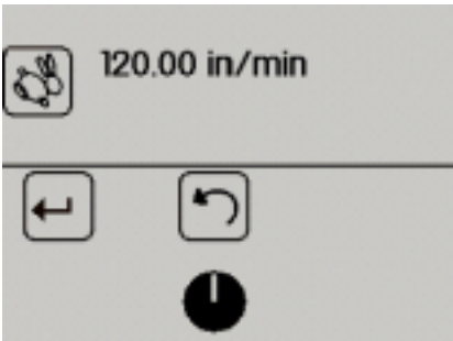
Figure 4: Setup screen for travel speed while welding.
