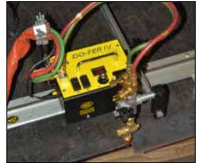
Shown above, oxy-fuel setup of Go-fer IV
