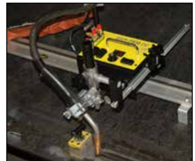
Shown above, welding setup of Go-fer IV
