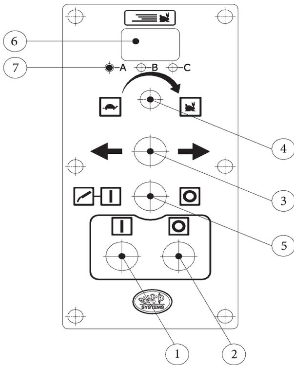
1. **Cycle Start Button** - Push button to initiate weld cycle. Weld contact will close, according to time settings, if the Weld Switch is set to Auto, the carriage will travel in the direction selected by the Travel Direction Switch.
